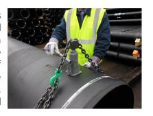
DO NOT USE EXCESSIVE FORCE OR EXTENDED MEANS TO CREATE UNSAFE LEVERAGE OR STRAIN UPON THE JACK OR CHAIN.
