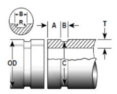
**"A" Dimension** - The "A" dimension, or the distance from the pipe end to the groove, identifies the gasket seating area. This area must be free from indentations, projections, deep pits and swells from the pipe end to the groove to provide a leak-tight seal for the gasket.
