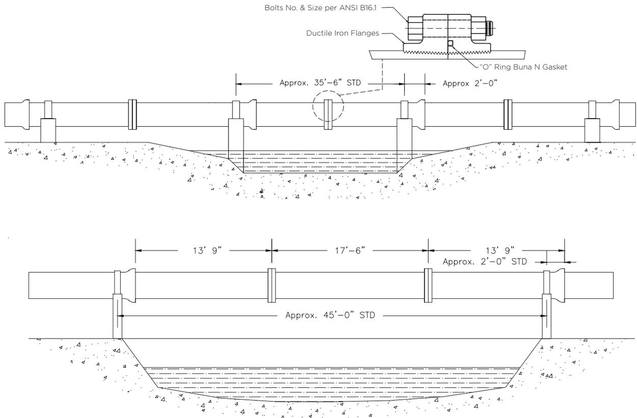
Long-Span Pipe is a Ductile cast iron multiple length pipe using a unique O-Ring Rubber Gasket Joint designed by McWane Ductile to minimize the number of piers required in elevated lines. Installation requires support under each bell, with allowance for expansion and contraction. The length tolerance of each unit is plus or minus 1/4 inch. Pipe are shipped unassembled, with accessories packaged separately. The pipe
