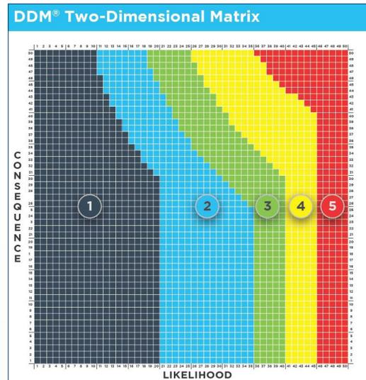
Once the consequences and likelihood values are totaled, the two values can be used to plot the intersecting point on the DDM® graph. The color-coded recommendations table provides specific recommendations.
