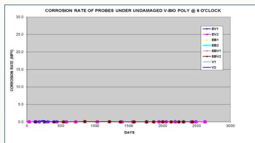
As effective as traditional polyethylene encasement is, the graphic comparisons above illustrate the improved performance of V-Bio® under the same severely corrosive conditions.
