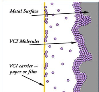
Loosely bonded hydrogen molecules on the metal surface control corrosion until they are dislodged by corrosion processes driven by dissolved oxygen molecules. VCI molecules are attracted to the surface to produce a strong polar bond, hydrogen film, thereby regaining control of the corrosion processes.
