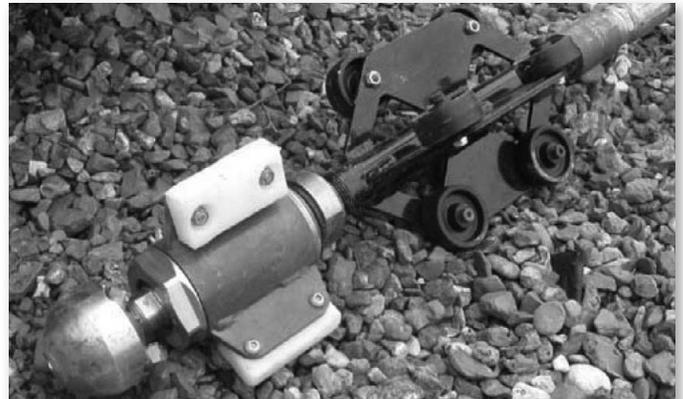
Photo shows Vactor Blue Twister Nozzle and appropriate assembly. Photo provided by the Ductile Iron Pipe Research Association.
